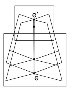
Epipole has same coordinates in both images. Points move along lines radiating from e: "Focus of expansion"
