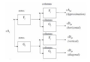
Figure 1: Stationary Wavelet Transform (SWT)
