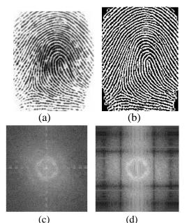
Figure 4: (a) original Image (b) enhanced Image (c) and (d) Fourier Spectrum of (a) and (b) respectively.
