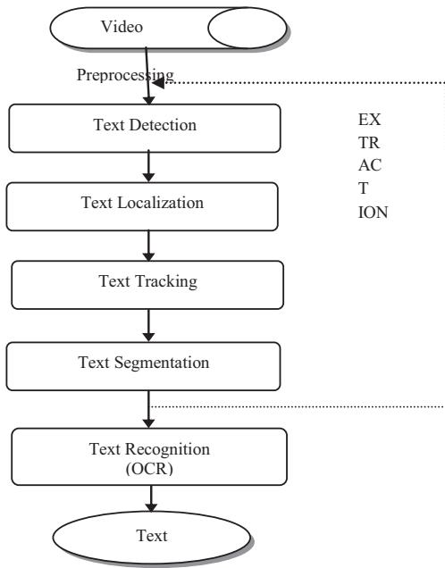
Figure 2.System for character detection and recognition from video/image
