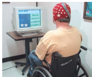
Figure 4. Example of an EEG-based BCI platform. Notable elements include the electrode cap worn (asterisk) by the subject and the viewer screen (double asterisks) for which the subject controls the cursor on the screen (BCI computer not shown) by various EEG signals and signal processing methods (i.e., sensorimotor rhythms, SCP, or P300 paradigm)
